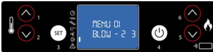
2. Pressing the SET key to access the menu to set the speed of your canalisation fan.
