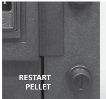
**Pellets temperature safety:** In the rare event there is a too high temperature in the tank, the thermostat for pellets safety with manual reset creates an alarm **"ALAR-SIC-FAIL"** stopping the pellet stove. You need to reset the system working on the device placed on the back of the stove.
