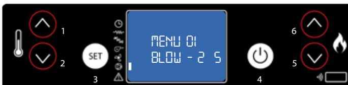
4. To turn off the fan of the canalization, set the speed to 0.
