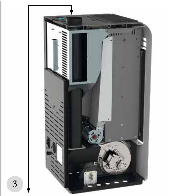
Break the pre-cut top and vertically connect the smoke pipes until the top of the stove. It is strictly necessary that the smoke pipes wouldn't be in contact with pellet tank, ensuring the correct passage of air between smoke pipes and pellet tank.
