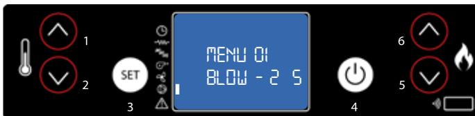
3. Set the speed using the button 1. With key 1 you set the speed of the fan.
